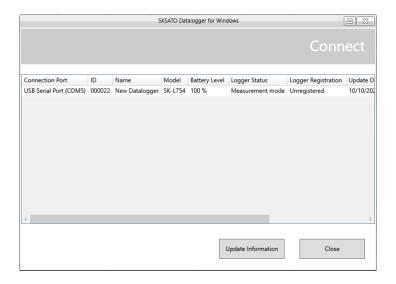
5) Connection is complete. Configure the datalogger via the software at your preference.
